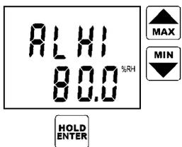
It is possible to leave the alarm setting mode by pressing MENU key. New adjusted limits up to pressing MENU key are stored in memory. After pressing ENTER key it is possible to set alarm limits for dew point temperature.
