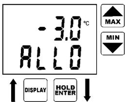
Reading ALLO indicates adjusted lower alarm limit (here air temperature). Set the desired value by means of the arrow keys. Press and hold the arrow key UP to make value increase fast. Press and hold the arrow key DOWN to make value decrease fast. Release the arrow key and press ENTER to confirm new limit.
