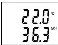
Temperature in °C is displayed on the upper LCD line and relative humidity in %RH is displayed on the lower LCD line.
