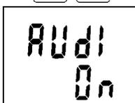
This item indicates if audio signaling of alarm indication is switched on (On) or switched off (OFF). Press ENTER key to change actual setting.
